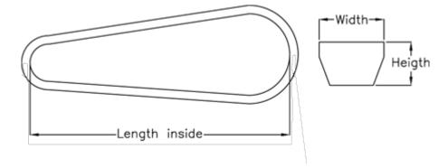
$\begin{array}{ll} \text{Datum Llength} = 925 \\ \text{Height} &= 8 \\ \text{Length inside} &= 900 \\ \text{Width} &= 13 \end{array}$
